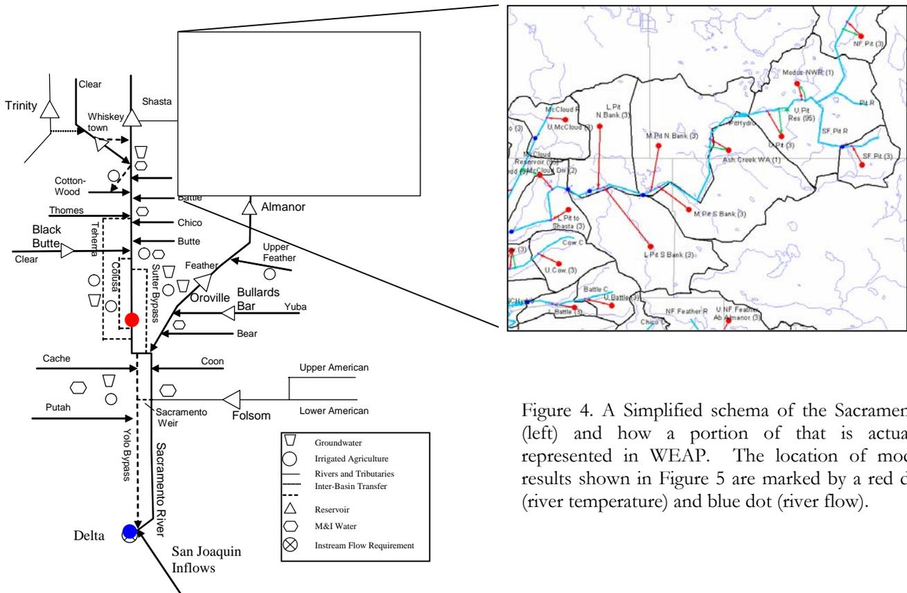
Figure 4. A Simplified schema of the Sacramento (left) and how a portion of that is actually represented in WEAP. The location of model results shown in Figure 5 are marked by a red dot (river temperature) and blue dot (river flow).
